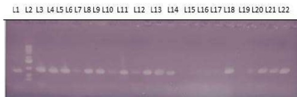
Figure 2: PCR assay results of 20 field samples. L1: Positive control L2: Ladder L3 to L22: Field samples Positive samples are- 15: L3, L4, L5, L7, L8, L9, L10, L11, L12, L13, L14, L18, L20, L21, L22 Negative samples are- 5: L6, L15, L16, L17, L19
