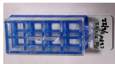
Figure 1: Lab-Tek™ Chamber Slide System for growing cells on a standard microscopic slide for on-spot visualization after staining
